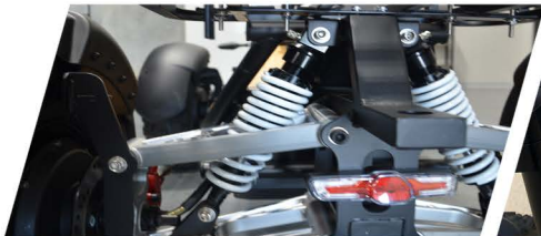
4 WHEEL INDEPENDENT SUSPENSION Each Wheel Moves Independently For Improved Handling & Comfort On Almost Any Terrain.
