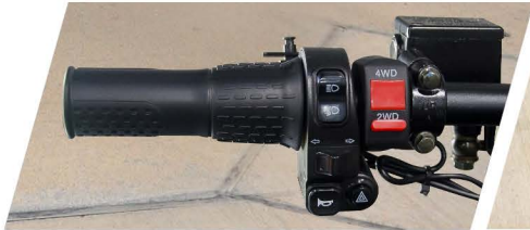
ALL WHEEL DRIVE SWITCH 2WD / 4WD Easily Engage A.W.D. For Maximum Traction For Challenging Conditions & Tough Terrain.
