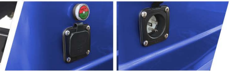
3 PRONG ONBOARD CHARGING PORT Standard 3-Prong Port - Heavy Duty Extension Cable Not Included.
